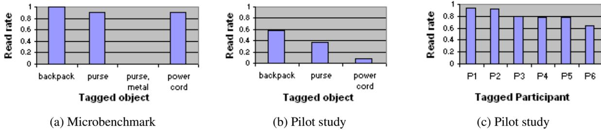
Figure 3. Read rates for tags in a laboratory benchmark and in the pilot study
